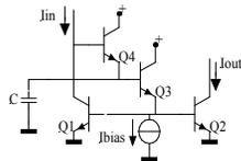
Fig. 4b. Peak detector circuit.
