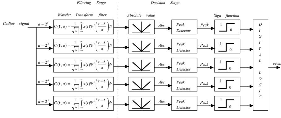
Fig. 2. Block diagram of the wavelet system
