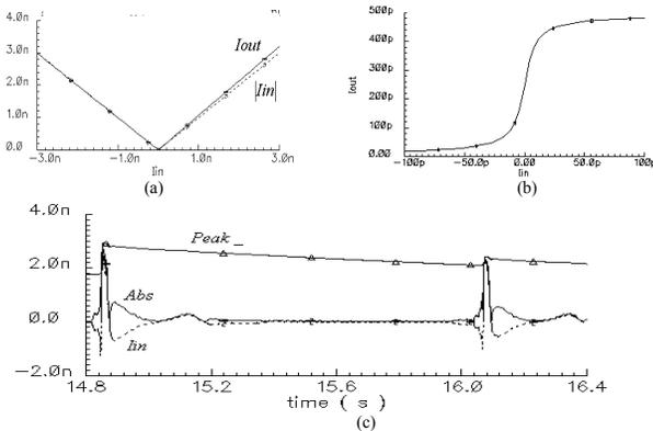
Fig. 7. (a) DC Response of the absolute value circuit (b) DC Response of the comparator (c) Transient response of the absolute value and peak detector circuits with a ventricular signal at the input.
