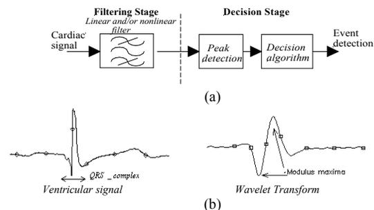
Fig. 1. (a) Block diagram of the basic structure of the QRS detectors [4]. (b) Cardiac signal and the modulus maxima of the WT
