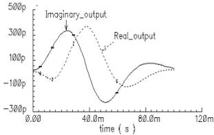
Fig. 6. Impulse response with 3 CFOS stages
