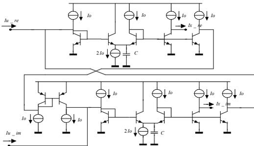
Fig. 3. Equivalent DTL circuit for complex input for the analog CFOS stages.
