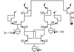
Fig. 5. Comparator circuit.
