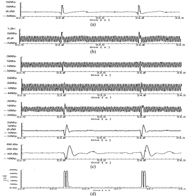
Fig. 8. (a) Ventricular signal (b) Ventricular signal with 50Hz interference (c) the wavelet transform at five subsequent scales (d) QRS complex modulus maxima detection for  $j=4$ .
